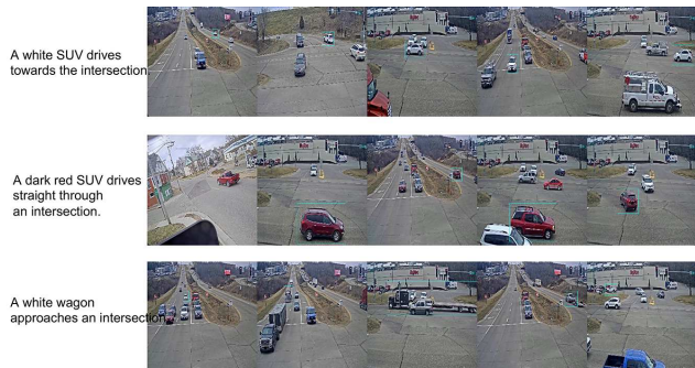
Figure 4. Examples of five highest matching images for each NL description. The NL description is on the left, and the images are sorted in descending order according to the matching probability on the right.
